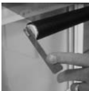
FIG 7: Wind spring clockwise
