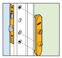
**2.** Loosen interior face plate screws, and remove interior and exterior face plates.
