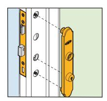
4. Align funnels on exterior face plate with screws, insert deadbolt spindle into key cylinder, and loosely finger-tighten the screws.
