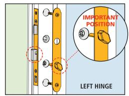
**3. With deadbolt extended and deadbolt knob in position shown,** insert deadbolt spindle through lock body, and insert interior face plate screws through door.
