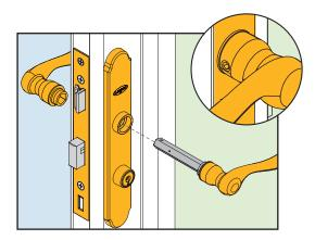
Open door and use deadbolt knob to extend deadbolt. Loosen handle set screw with the Allen wrench provided, and remove interior and exterior handles.
