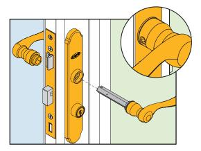
**5.** Insert handle spindle through lock body and into opposite handle. Tighten set screw with Allen wrench. Tighten interior face plate screws.
